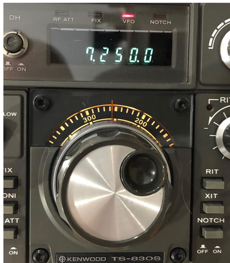
Figure 15- mechanical dial discrepancy
