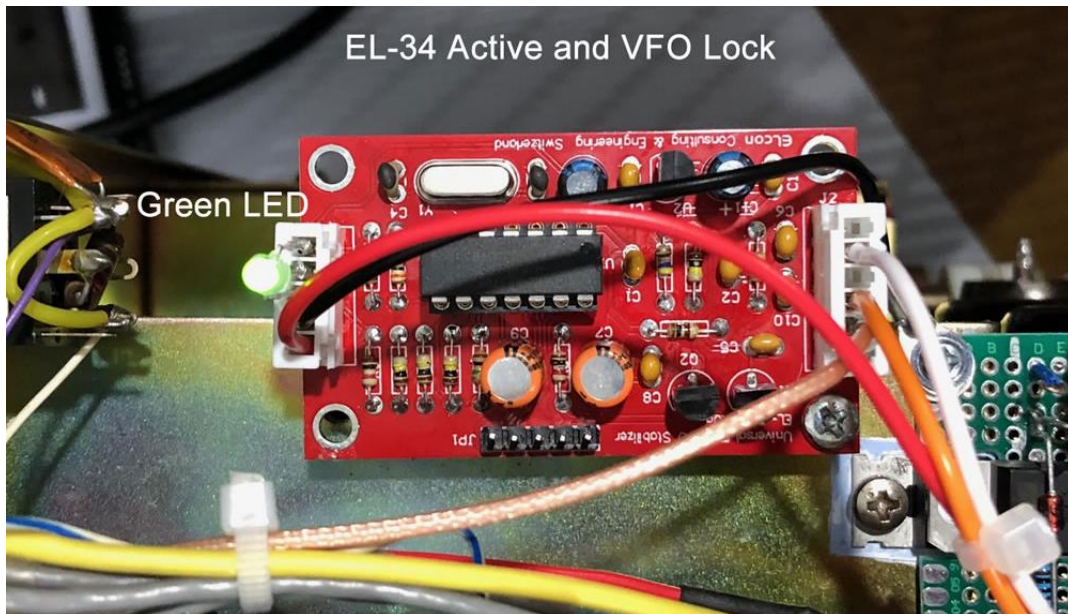
Figure 14- green LED to indicate VFO lock
